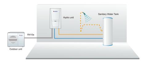
Heating / Cooling with Water Heating
