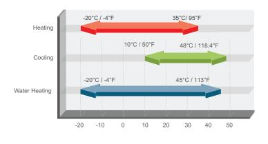
Heating - Fan Coil/Radiator:  $25^{\circ}$ C  $\sim 55^{\circ}$ C ( $77^{\circ}$ F  $\sim 131^{\circ}$ F) Floor:  $25^{\circ}$ C  $\sim 45^{\circ}$ C ( $77^{\circ}$ F  $\sim 113^{\circ}$ F) Cooling - Fan Coil/Radiator:  $7^{\circ}$ C ~  $25^{\circ}$ C ( $45^{\circ}$ F ~  $77^{\circ}$ F) Floor:  $18^{\circ}$ C ~  $25^{\circ}$ C ( $65^{\circ}$ F ~  $77^{\circ}$ F)
