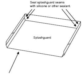
Open end of splashguard should rest on the horizontal drain pan.
