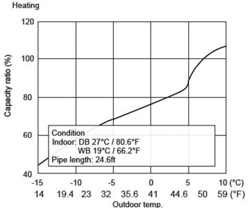
Figure 5: 18/24K Capacity ratio vs outdoor temperature
