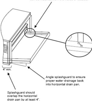
Figure 22: Splashguard with front slope
