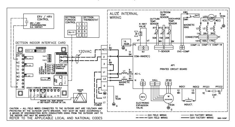
Figure 15: 24K Electrical diagram
