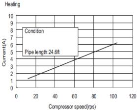
Figure 3: 18/24K Operation characteristics curves
