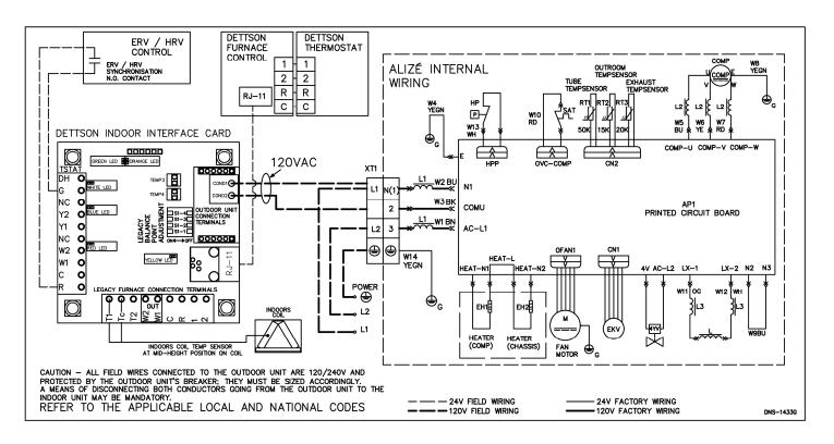
Figure 14: 18K Electrical diagram
