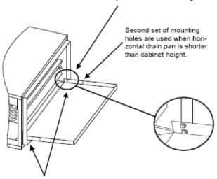
Fasten splash guard to duct flanges with (4) sheet metal screws. (2) on each side. Screws can be installed from the inside or outside.
