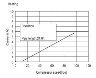
Figure 2: 12K Operation characteristics curves
