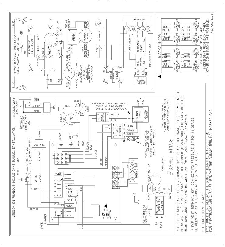
Figure 11: Wiring diagram variable speed motor (ECM)
