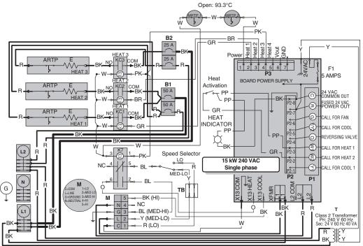
For the use of a two-stage thermostat or an outdoor thermostat, connect between W1 and W2. Make sure that the Heat Activation switch is set to "Slow" position.
