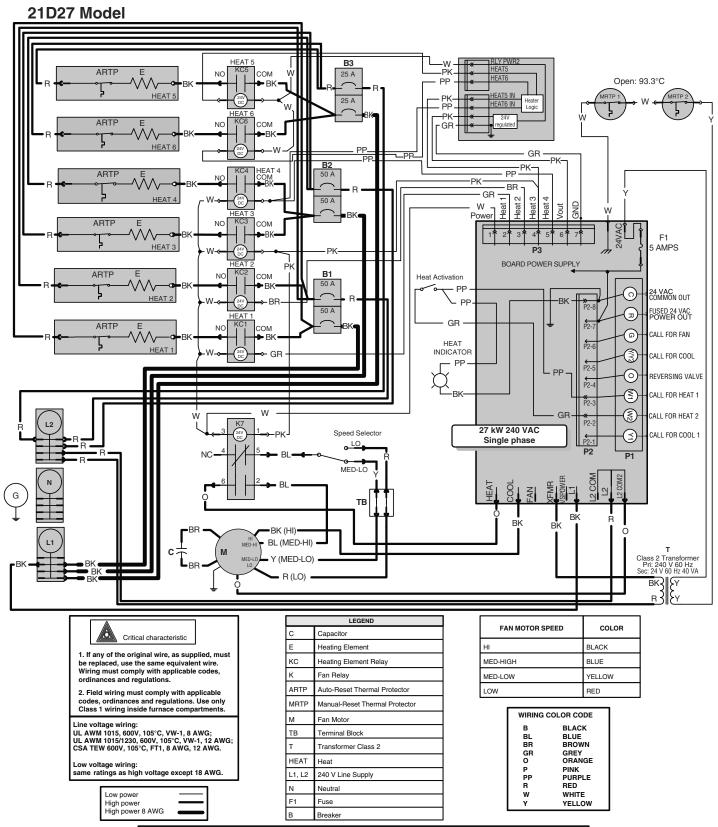
For the use of a two-stage thermostat or an outdoor thermostat, connect between W1 and W2. Make sure that the Heat Activation switch is set to "Slow" position.
