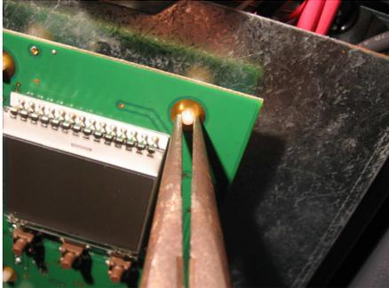
3. Disconnect the defective control board
