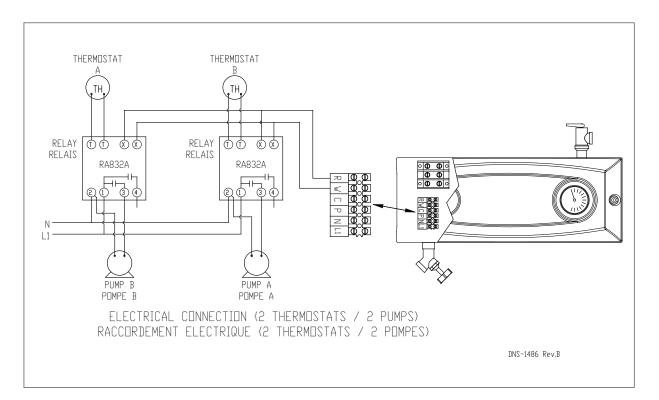
Figure 5 – Multi-zone Diagram with more than one Circulator
