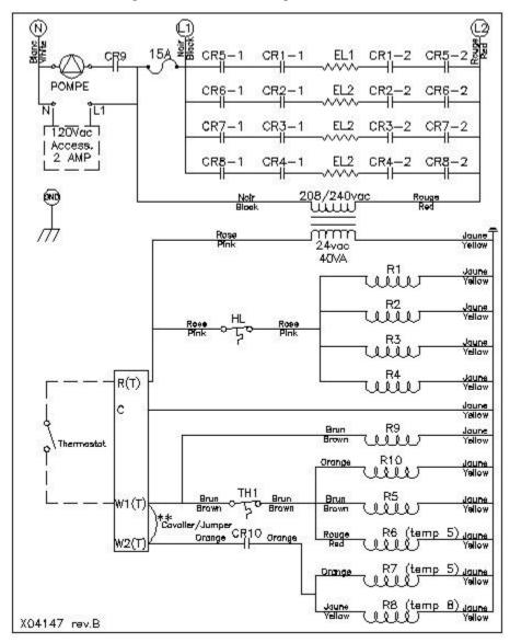
Figure 7 – Electrical Diagram 4 elements
