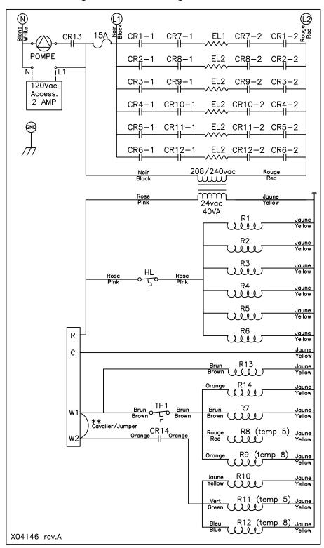
Figure 8 – Electrical Diagram 6 elements
