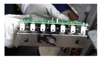
16- Place the assembly on the tank, the bolts in the middle of the holes
