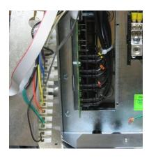
8- Move the protection plate to the left of the machine in order to access the power board
