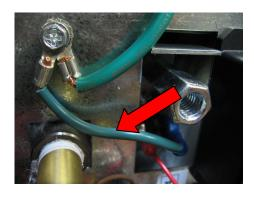
12- Unplug the black wire connecting the relay to the power board
